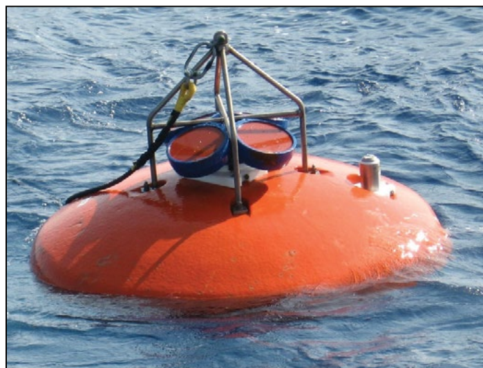
Teledyne RDI ADCP in Top Buoy of LOCO Mooring.
