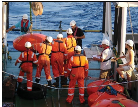
Ellipsoidal flotation collars are prepared for deployment on LOCO moorings.
